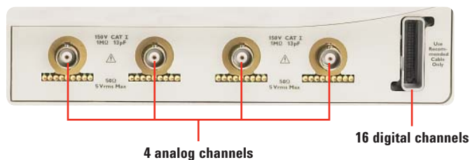
Figure 25. Analog and digital channels on an Agilent MSO 8000 Series oscilloscope
