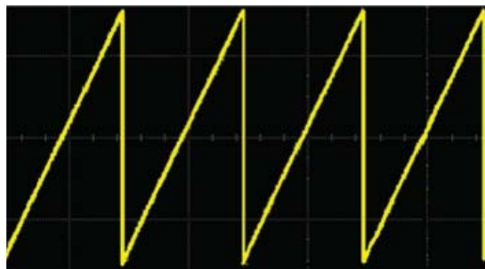
Figure 6. A sawtooth wave
